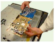
5. Separate the M/B and D-tuner board.
