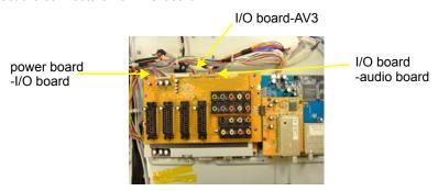
2. Remove the four screws securing the I/O board and four screws securing the A-tuner board.
