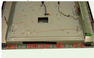
4. Remove the PCD chassis as shown.
