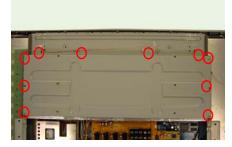
2. Push the top shielding a little bit upward.
