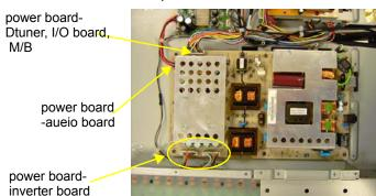
2. Remove the 9 screws securing the power board and remove the power board.
