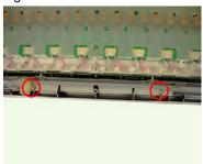
2. Remove the two screws on the left.
