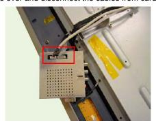
4. Disconnect the cables from AV3 board.
