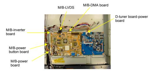
2. Remove the four nuts and two screws securing the mainbaord.
