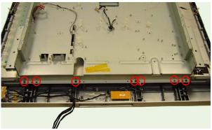
3. Remove the 10 screws on chassis top view.
