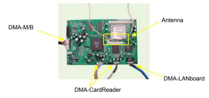
2. Remove the six screws securing the DMA board and remove it.
