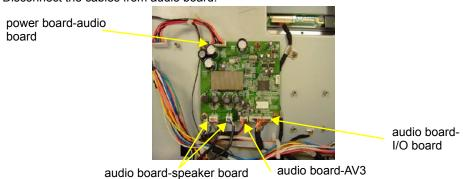
2. Remove the four screws securing the audio board.
