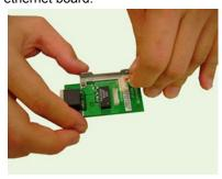
4. Remove the two screws securing the ethernet bracket and remove the bracket.
