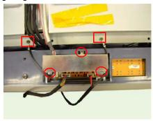
3. Turn the card reader module over and disconnect the cables from card reader module.
