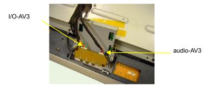
**5.** Remove the two screw securing the AV3 board and remove it from card reader module.
