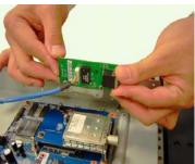
3. Disconnect the cable from the ethernet board.
